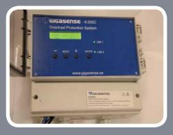
Gigasense 9:302C Electronic Unit for overload protection
