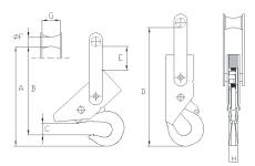
The Automatic Hook is available in 6 sizes from 2 to 27 tons. It is easy to operate, has rugged design and a high reliability.
