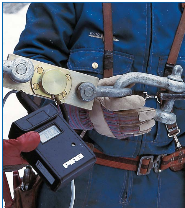
Here the PIAB LL Link and PIAB Instrument are used when weighing engine parts.
