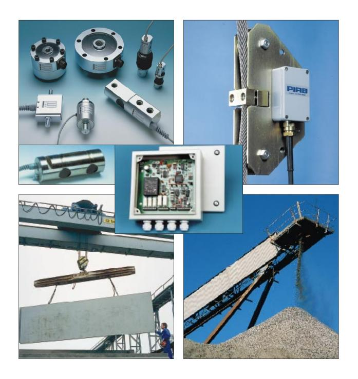
PIAB Electronic Units 9:300/9:400 for overload guards. Advanced units that are capable of processing signals from different types of power transducers. Eminently suitable for protecting lifting devises, conveyors, machinery, etc. against overload. Output functions are available as potential free contacts and output signals for load indication.
