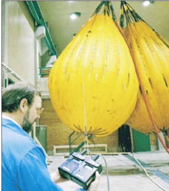
Testing overload guards at a paper mill by means of water weights. The reading is taken by a PIAB Remote Read-Out Instrument.
