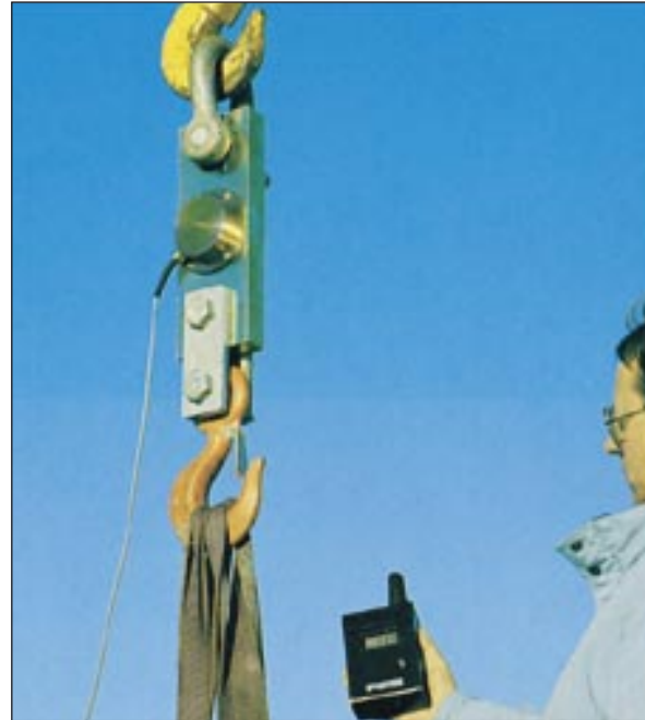
Here the PIAB LL Link and Instrument are used when weighing engine parts.
