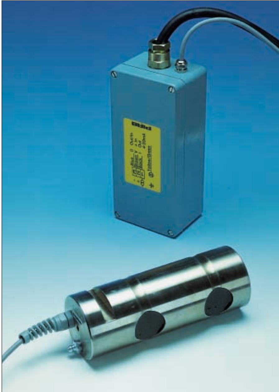
The PIAB Load Pin can be dimensioned to replace an existing shaft. The PIAB Load Pin/ Transducer Amplifier are compatible with all PIAB electronic systems for over-load protection and load indication. The PIAB SLC and PIAB LCA are made for use in aggressive environments and fully conform to IP 67.
