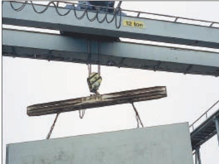
*PIAB Load Pin SLC mounted in an equalisation sheave.*
