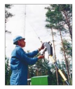
Also when stay ropes are difficult to reach the light-weight RTM 20D is easy to handle. The picture shows control of guy wire tension from a crane operated working platform.
