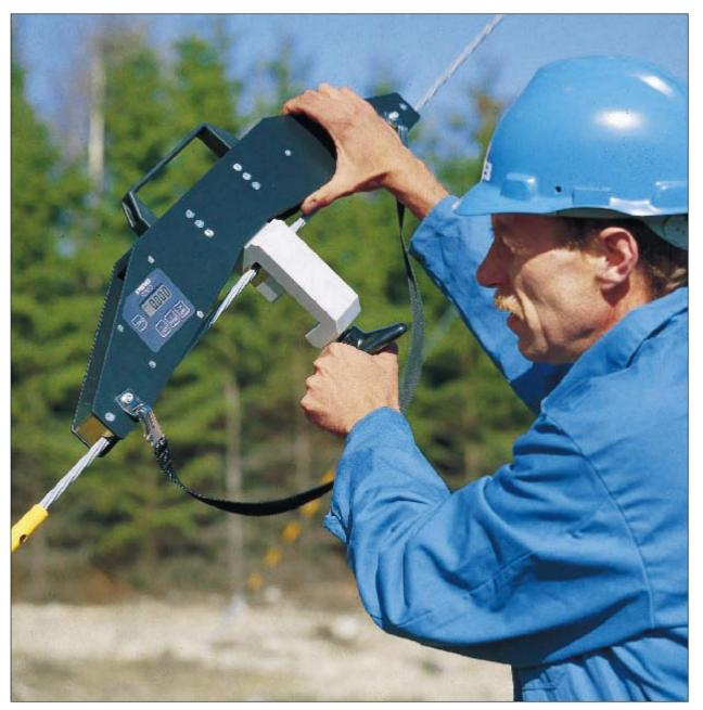
The RTM 20D can be used in applications where accurate measurement in pre loaded wire ropes is required. Such applications can be stay ropes, suspension ropes, catenary ropes etc. The RTM 20D is applied direct to the rope and the measured tension value is presented digitally.
