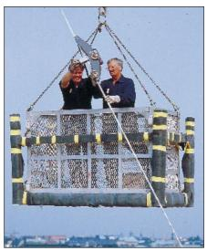
The PIAB RTM 20D is in use when installing/inspecting suspension and catenary ropes.
