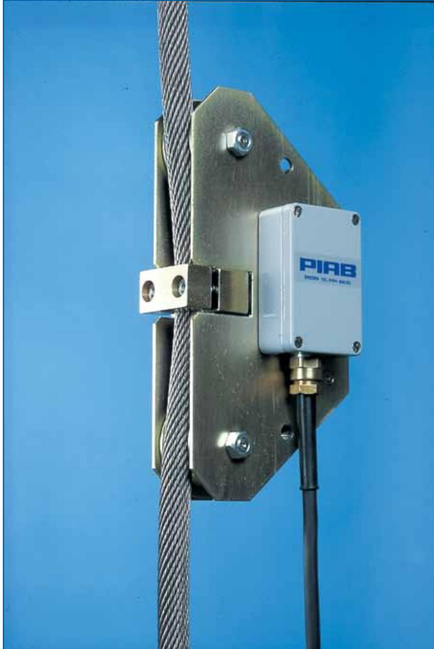
The PIAB LKVE is a force transmitter which is attached to a stationary rope part. PIAB LKVE gives a 4-20mA output signal. It has high repeatability, is made for use in aggressive industrial environments and fully conforms to IP 67.
