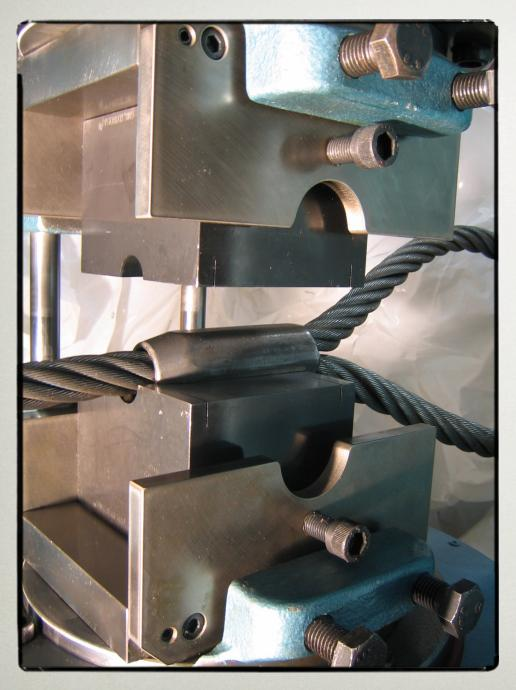
The One Press® Swaging System consists of the unique combination of One Press® Sleeves and One Press® Dies.
