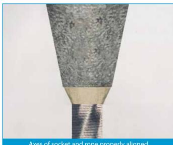
Axes of socket and rope properly aligned and sealed with plasticine (Fig 4)
