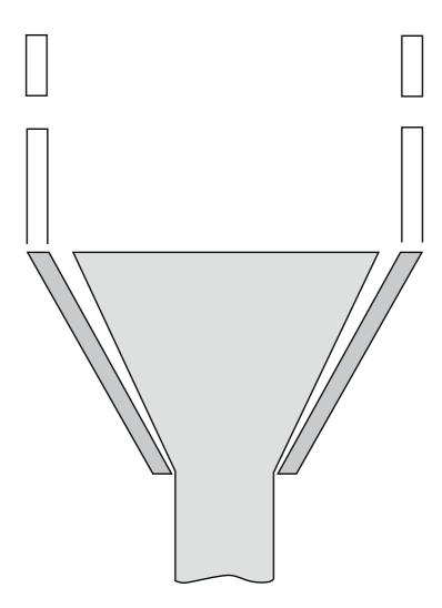
Exaggerated Relationship between Cone and Socket after the Resin has cured Figure III
