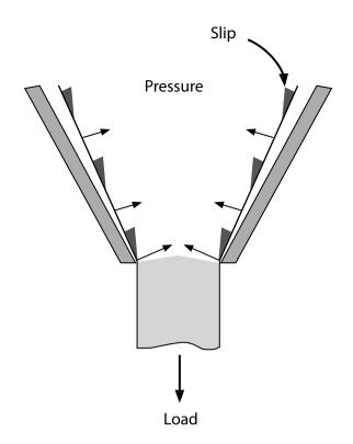
Load causes the cone to slip at the socket interface and the pressure generated locks the cone within the socket
