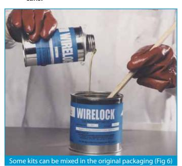
6.5 Only the 100cc, 250cc & 500cc can be mixed in the original packaging by pouring the resin into the granular materials container. In the case of other kits, a proper mixing vessel should be used (Fig 6).
