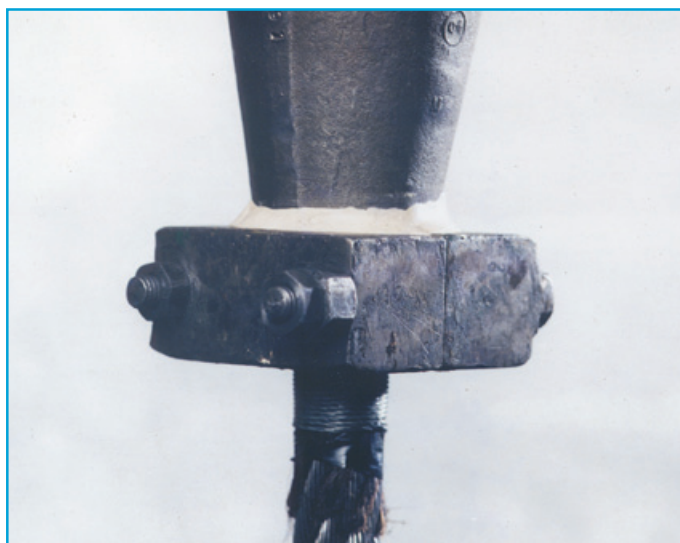
Clamp used to align rope and socket before sealing with plasticine (Fig 5)
